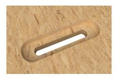
Available on any parapet cap configuration the oblong countersunk holes accept 1/2" (13 mm) diameter concrete anchors with up to a 1 1/4" (31.75 mm) washer. The oblong design is used primarily when "wet-setting" your anchors and are placed 24" (610 mm) on center and 6" (152 mm) from the ends of the 16' (4.8 m) board.
